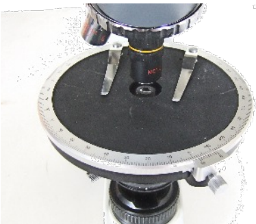
Large 360° rotating graduated stage, stage clips and locking screw
