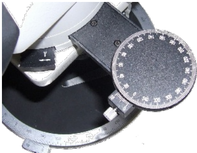
Push-in analyser (360° rotating) and 1st order red tint
