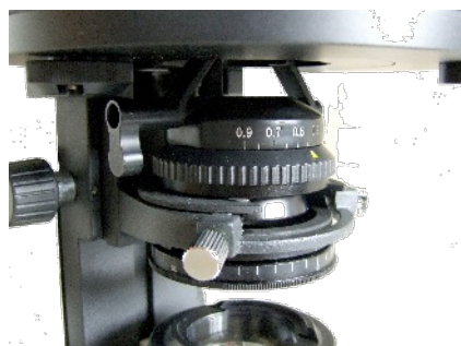
NA 0.9 condenser with flip-in lens and integral rotating polariser
