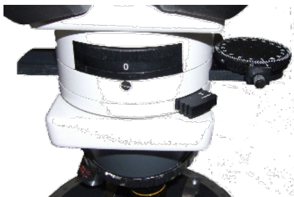
Analyser, 1st order red tint plate and bertrand lens
