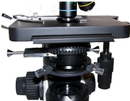
Condenser NA 0.9 with phase slider inserted.
