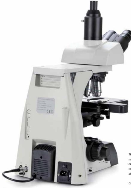
The carrying grip at the back of the microscope ensures safe transportation of the microscope and the integrated tool & holder make sure the right tool is always available
