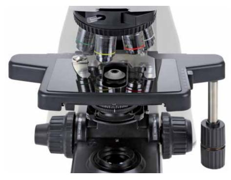
Optional: mechanical stage with scratch-resistant Sapphire glass
