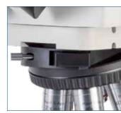
For slider with  $1\lambda$  retardation plate for observation of monosodium crystal deposition (gout) and for DIC slot (DIC ready)
