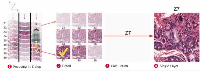
High Precision - Used for flatness slide or requirement for high precision image
