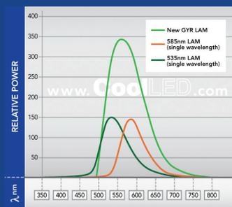
Recent developments in LED technology have enabled increased intensity in what was historically the weaker green-yellow-red ("GYR") region of the LED spectrum. A new wide spectrum GYR LAM is now available and can readily be fitted to new and existing pE-2 systems. The graph shows the greater comparative intensity of this LAM over the previous LED wavelengths available for this spectral region.
